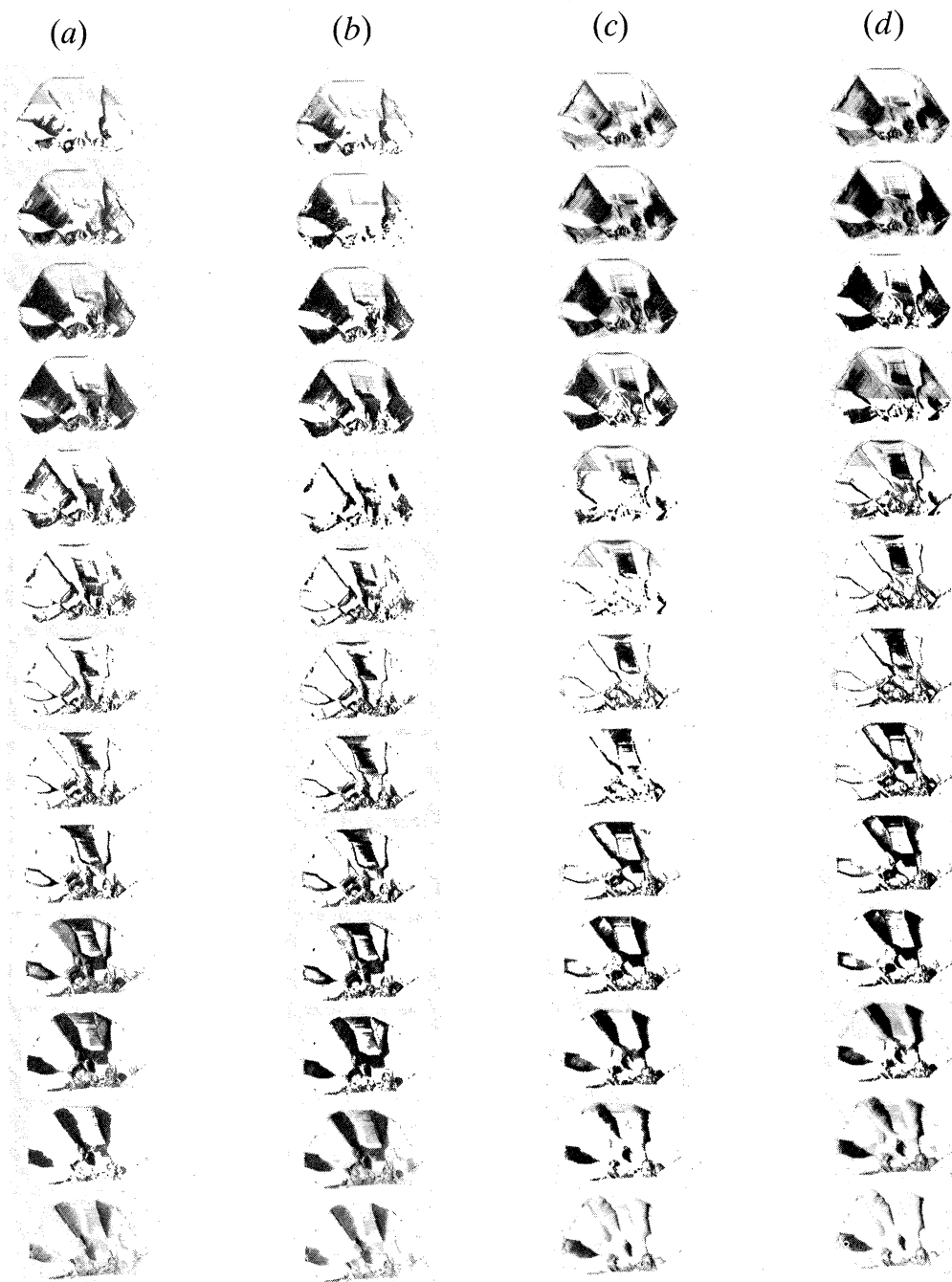
Figure 10. Sequences of double-crystal topographs recorded with 2\theta_M = 150^\circ , \lambda = 0.121 \text{ nm} , \omega increasing in nominal 1 arcsec steps from top to bottom. Recorded on Agfa-Strukturix D7 film, exposures ca. 70 mA minutes. (a) \chi = 180^\circ , diffraction geometry similar to figure 9, but view of specimen surface less oblique (film 1*). (b) Repeat of (a) (film 5*). (c) \chi = 0^\circ , image rotated 180^\circ in its own plane for comparison with (a) and (b), so that the specimen viewing direction is from left of the surface normal (film 1). (d) Repeat of (c) (film 5).
